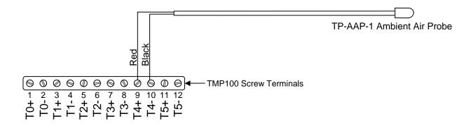
Figure 1 - Wiring Diagram
